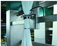
In the quickest way possible the tubular fabric is disentangled, opened and dehydrated by passing the ring suction nozzle. The fabric is dehydrated across its entire circumference in a very even, gentle and effective way.
