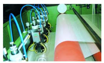
SUCUT-Cutting machines are perfectly suited for longitudinal and lateral cutting of different quality fabrics. Depending on the type of material and its composition several different cutting processes such as blade, pinch and ultrasound cutting, as well as different tools such as beating blades, tape blades or circular blades can be used.
